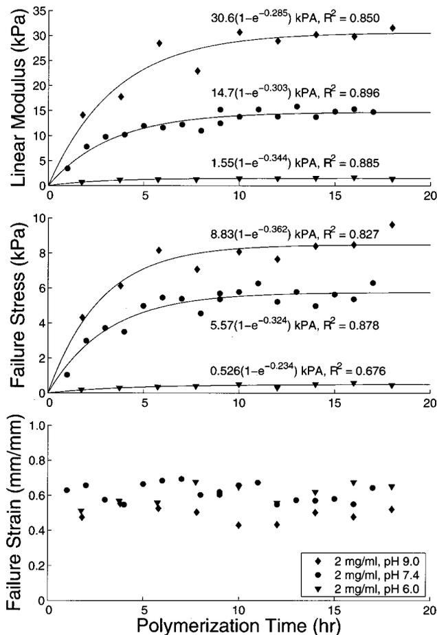
**Fig. 9** Effect of polymerization time on the linear modulus, failure stress and failure strain of pH 6.0 (▼), pH 7.4 (●), and pH 9.0 (◆) collagen matrices (2.0 mg/mL) tested at a strain rate of 38.5 percent/min. Exponential curve fits are shown for the linear modulus and failure stress data.
