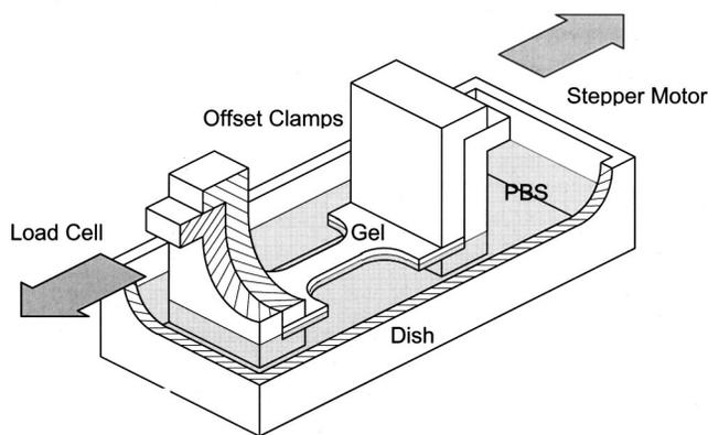
**Fig. 2 Cut away view of the experimental setup used for mechanical testing of collagen matrices. Collagen matrices were tested while submerged in PBS, pH 7.4 at 37°C.**
