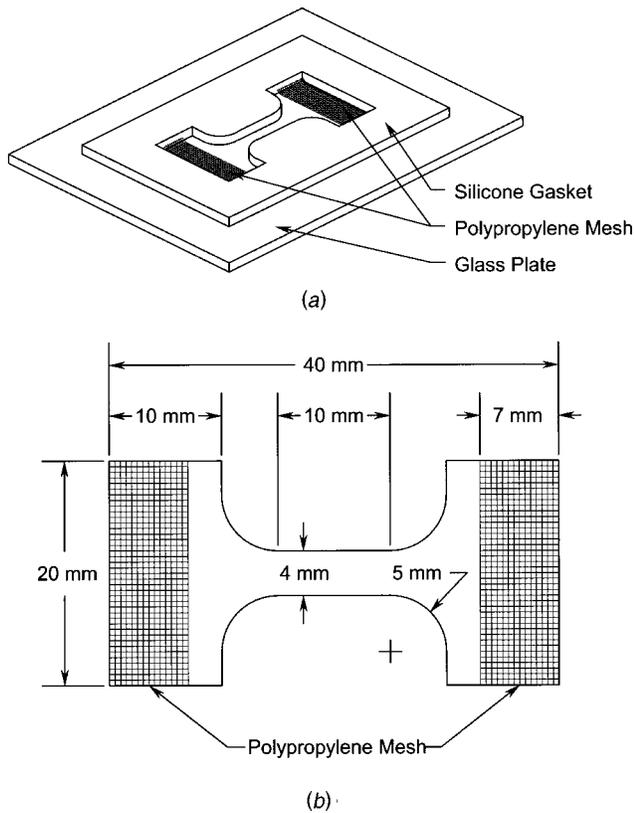
**Fig. 1 Construction of the mold used to prepare collagen matrix test specimens (a). Schematic showing the dimensions of the collagen matrix test specimen with polypropylene mesh reinforcement (b).**
