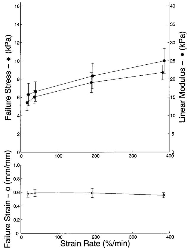
Fig. 12 Effect of strain rate (19.2–385 percent/min) on the linear modulus (●), failure stress (◆), and failure strain (○) of collagen matrices (2 mg/mL, pH 7.4)
