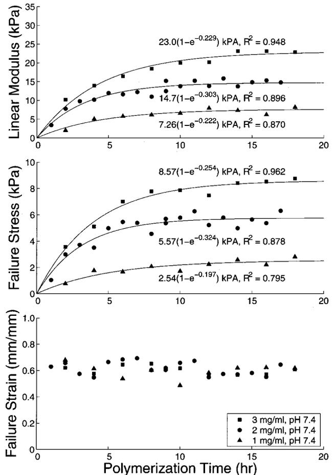
**Fig. 8** Effect of polymerization time on the linear modulus, failure stress and failure strain of 1.0 mg/mL (▲), 2.0 mg/mL (●), and 3.0 mg/mL (■) collagen matrices (pH 7.4) tested at a strain rate of 38.5 percent/min. Exponential curve fits are shown for the linear modulus and failure stress data.
