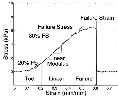
**Fig. 3 Representative stress-strain curve of a collagen matrix (2 mg/mL, pH 7.4) tested at a strain rate of 38.5 percent/min. The stress strain curve can be separated into three distinct regions designated “toe,” “linear,” and “failure.” Determinations of linear modulus, failure stress and failure strain are demonstrated.**
