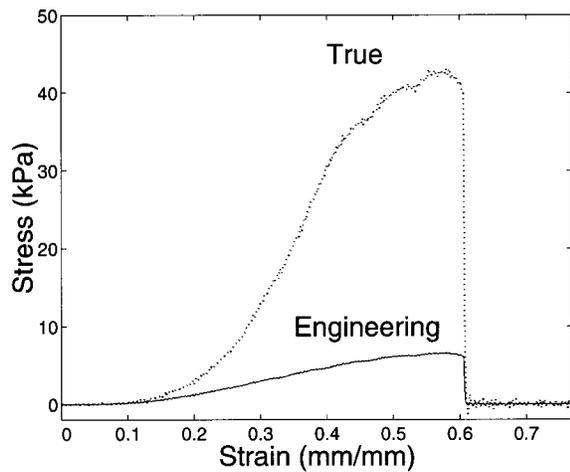
**Fig. 13 Comparison of “true” stress (approximated) and “engineering” stress (calculated) as a function of strain for a collagen matrix (2mg/mL, pH 7.4)**
