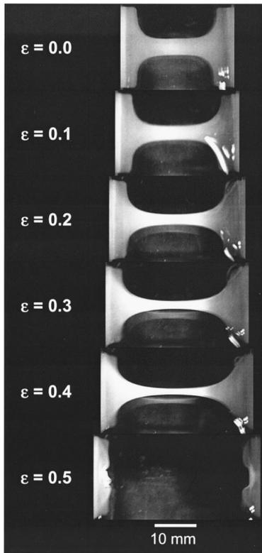
**Fig. 7** Time-lapse images demonstrating the tensile testing of a collagen matrix (2 mg/mL, pH 7.4) at a strain rate of 38.5 percent/min
