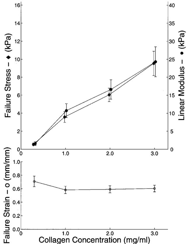
**Fig. 10** Effect of collagen concentration (0.3–3.0 mg/mL) on the linear modulus (●), failure stress (◆), and failure strain (○) of collagen matrices (pH 7.4) tested at 38.5 percent/min
