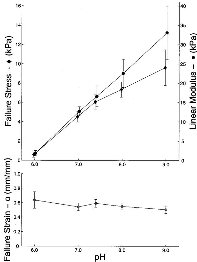
Fig. 11 Effect of phosphate buffer pH (6.0–9.0) on the linear modulus (●), failure stress (◆), and failure strain (○) of collagen matrices (2 mg/mL) tested at a strain rate of 38.5 percent/min
