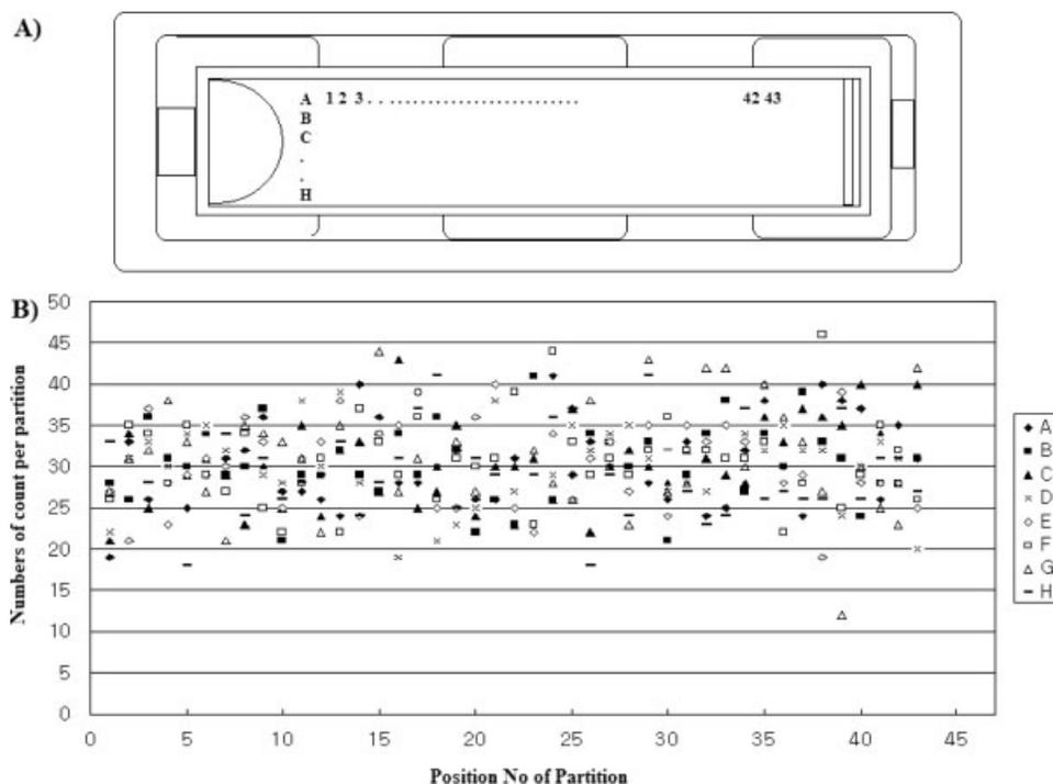
FIG. 1. The particle distribution pattern of microchip. (A) The microchip with divided partitions ( $43 \times 8$ ) for evaluation of even particle distribution. (B) The result of particle count in each partition.
