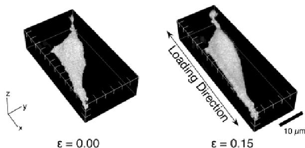
**Figure 10.** Three-dimensional reconstructed confocal images show deformation of a fibroblast within a three-dimensional tissue construct (collagen scaffold not shown) under unloaded and loaded (applied strain level of 0.15 mm/mm) conditions. To enhance discrimination of the cell from the surrounding collagen scaffold, cells were stained with the fluorescent membrane tracer dye DiOC<sub>6</sub>(3).
