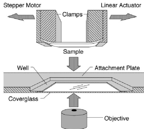
**Figure 2.** Schematic showing the interface between the mechanical loading instrument and the confocal microscope. An adapter plate provides the physical connection between the mechanical loading instrument and the confocal microscope and creates a well that allows specimens to be tested in an aqueous environment. Specially designed clamps offset the loading axis and hold the sample next to the coverglass.
