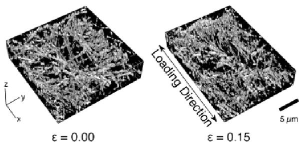
**Figure 4.** Three-dimensional reconstructed confocal reflection images show deformation of microstructure within a reconstituted collagen matrix (1.0 mg/ml type I collagen polymerized under physiologic conditions) under unloaded and loaded (applied strain level of 0.15 mm/mm) conditions.
