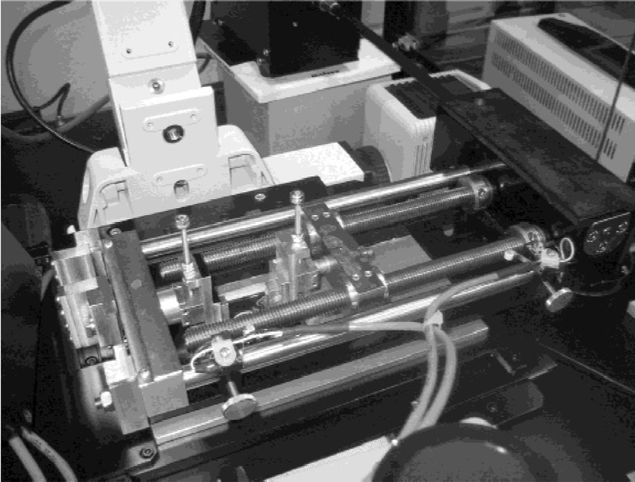
**Figure 1.** Photograph demonstrating the integration of a mechanical loading instrument with a laser scanning confocal microscope as a new means to perform microbiomechanical analyses of biomaterials and tissue constructs.
