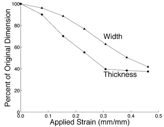
**Figure 8.** Width (▲) and thickness (●) measurements of a tissue-derived biomaterial at various levels of applied strain. Values are expressed as a percentage of original specimen dimensions (no applied strain).
