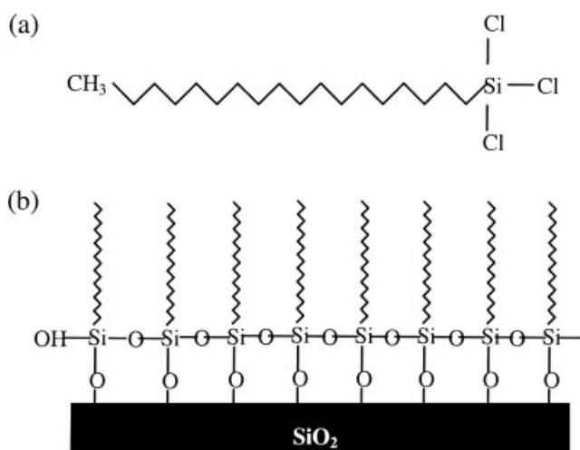
**Figure 1.** (a) Structure of octadecyltrichlorosilane (C<sub>18</sub>). (b) Possible structures of C<sub>18</sub> monolayer on the SiO<sub>2</sub> surface. (Drawing is not to scale.)
